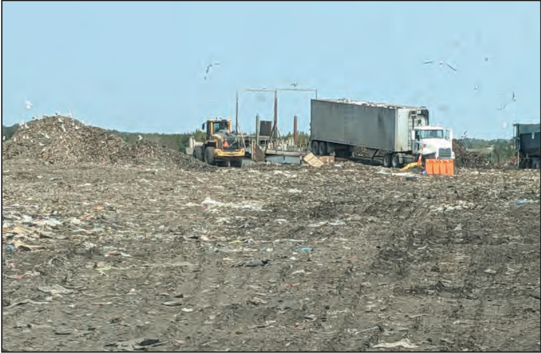
Tipper and active truck tipping, equipment clearing in front of tipper
